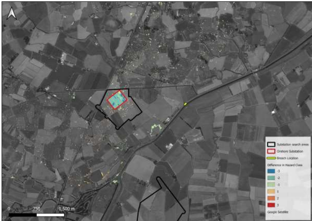
Figure 3-9 Hazard Class Changes Breach 2 - 0.1% AEP+CC
